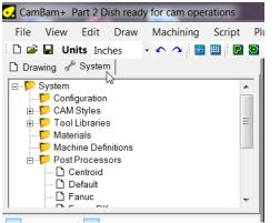
40. Click the + next to Post Processors to expand the list of post processors.
