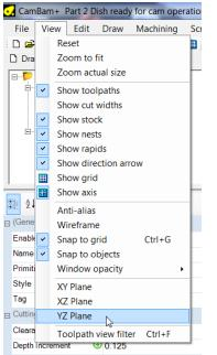
22. While you can generate machining operations in any view it will be easier to select them in our original top view or XY plane. To return to the top view, as before, select View→XY Plane.
