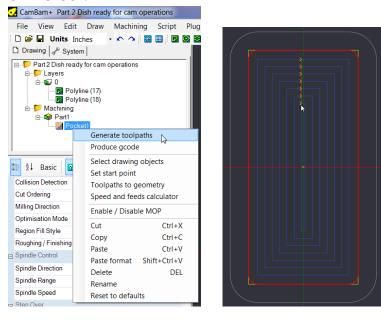
20. By holding the ALT key and the left mouse button we can rotate our view from 2d to 3d and see the depth of the passes we set above under the depth increment. Here there are 4 passes, this is especially visible below in the lower right corner by the mouse pointer. Visible here is also 2 vertical dashed red lines, these lines indicate where the bit will plunge and retract from each depth increment.
