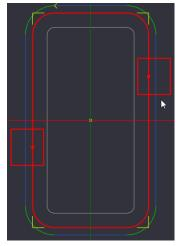
36. Since we have changed our tool path we need to again select Profile1 and select Generate Toolpaths to generate the tabs as shown below. Note where the mouse pointer is below and how it shows a blank space with retract and plunge moves where our two tabs will be located. These tabs will anchor our workpiece to the stock and prevent it from breaking free and damaging the bit or/and workpiece.
