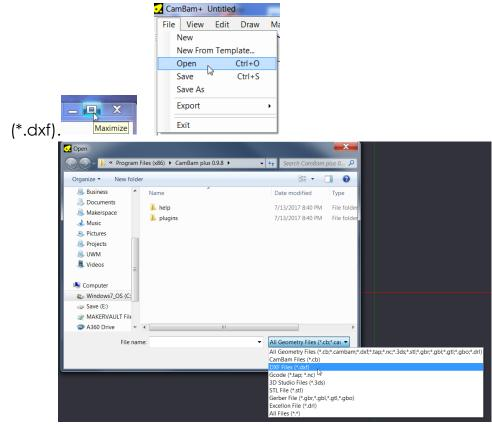
I'm Curious: While CamBam is able to import a .stl type file it can only be used for creating true 3d profiles. .stl can NOT be used to generate profiles, pockets, engraves, or drills, meaning you can not import a .stl from the internet for 3d printing into CamBam and cut it out on the router. The dish you will create in this tutorial is defined as 2.5d
