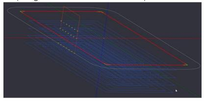
21. We can change our view to the side of the part by selecting View→YZ Plane. In the YZ plane the multiple depth passes and dashed plunge and retract lines are clearly visible.
