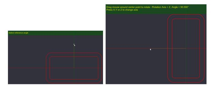
10. Select the small +(plus) sign next to 0. This expands the list of items in the drawing, instead of having 2 polylines (the inner and outer rectangle with rounded corners) in our drawing we have 16 separate items; this can be seen if we click on the part, instead of the whole line being selected each individual segment is selected, we do not want this.
