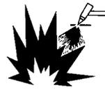
**FIRES AND EXPLOSIONS -- Heat from flames and arcs can start fires. Hot slag or sparks can also cause fires and explosions. Therefore:**
