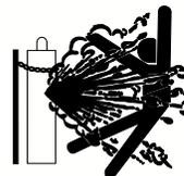
**CYLINDER** may explode if damaged. Keep cylinder upright and chained to support
