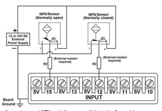
Fig. 6 Wiring diagram to connect NPN proximity sensors with internal pull up resistor.
