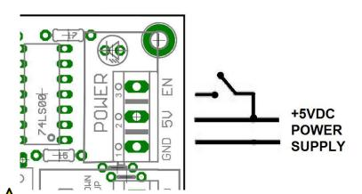
**WARNING:** This card must have the power supplied while it is connected to the PC. If power is removed to the card while it is connected to the PC, noise can be introduced to the output lines. This can create a dangerous situation as relays or other devices that might be connected to this card could get activated.
