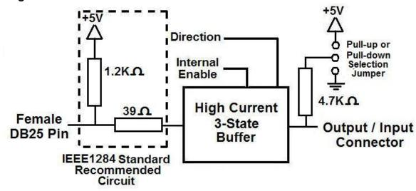
Fig. 1 Simplified functional block diagram for the 2-9 pins.
