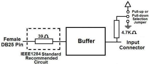
Fig. 3 Simplified functional block diagram for the inputs.
