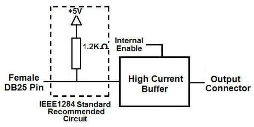
Fig. 2 Simplified functional block diagram for the outputs.
