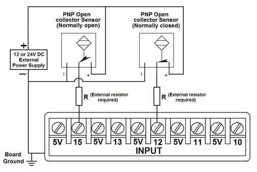
Fig. 7 Wiring diagram to connect PNP proximity sensors
