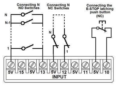
Fig. 3 Wiring diagram to connect switches.
