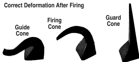
Correct Deformation After Firing
