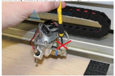
Instead use a short eyeglass type flat head screwdriver like this and adjust from the bottom of laser carriage:
